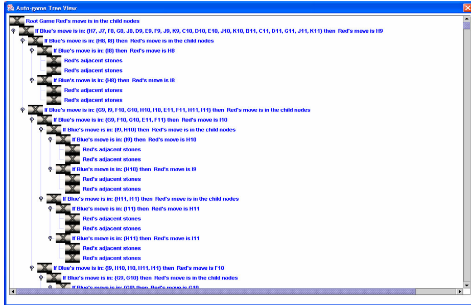
Fig. 9 A screen shot of the part of the tree derived by the MP deduction rule for the edge template of Fig. 6. The target T1 is at position I7 (see Fig. 8 for the coordinates). The depth of the tree is 11 and the number of nodes of 1008. The “Red’s adjacent stones” leaves correspond to adjacent cells (elementary strong connections).
